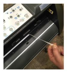
Before installing the new cutting strip remove the backing to expose the adhesive.
