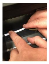
If you are installing a cutting strip on an older model cutter such as a 500-series, it may be necessary to take a flat object and run from one side of the strip to the other to ensure the strip is seated flat in the groove where the cutting strip sits.
