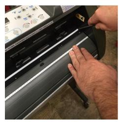
To replace the cutting strip on your BREN cutter, first we will need to power the cutter off and remove the old cutting strip. On either the right or left hand side of the cutting strip, use your fingertip or flat object to lift the cutting strip from the base of the machine.
