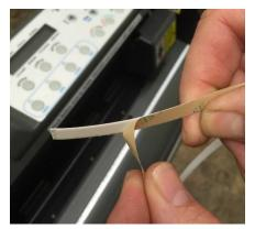
Starting from the left side of the cutter, place the new strip in the groove where the previous cutting strip was seated. Press the cutting strip flat in the groove until you reach the opposite side of the machine. There may be a small amount of cutting strip remaining that can be removed with a pair of scissors or a small utility blade.
